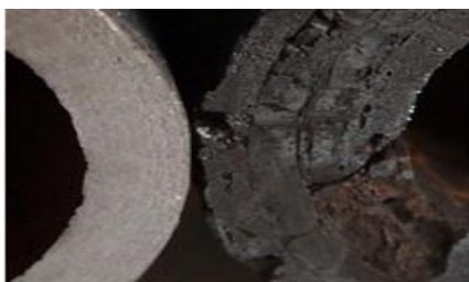
12Kh1MF steel before and after oxidation
